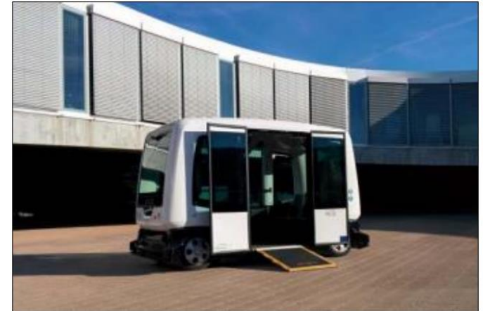
Figure 2 – EasyMile EZ10 with ramp for passengers with reduced mobility
