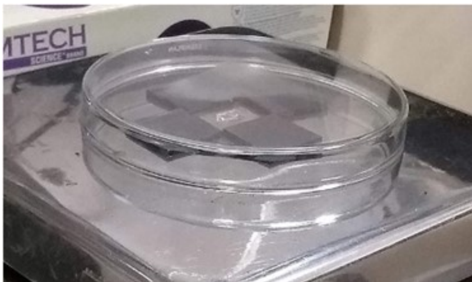
Figure F.1: Arrangement of perovskite films for solvent annealing. The microscope slide with 5 \mu\text{L} of 1.25 M MAI in DMSO is located at the center of the films.
