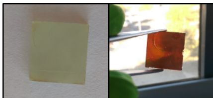
Figure 3.12. (Left) White solid formed on the substrate when the antisolvent is not added during the spin-coating step. (Right) MAPbI 3 perovskite film fabricated at ambient conditions.
