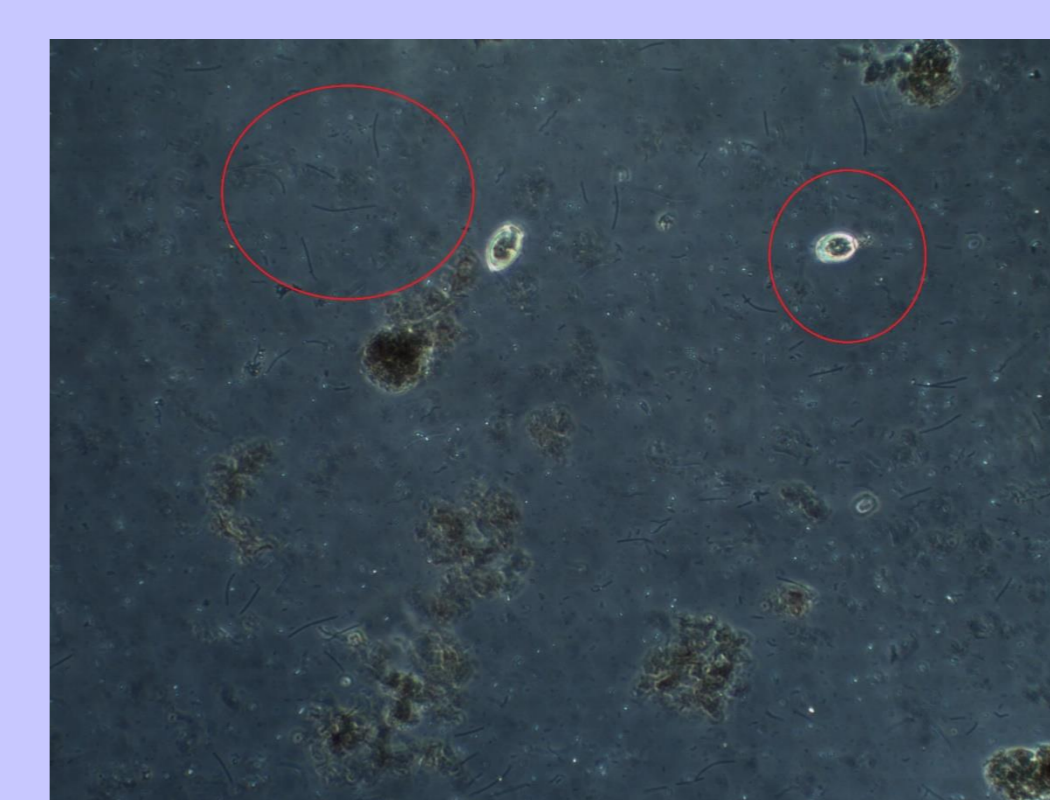
Waters, Ferric chloride pix 821- kemira + corn starch (0.2 \mu\text{l} + 0.075 \mu\text{l} ). Unknown mobile thick filament and Opercularia sp.
